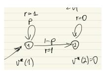
As can be seen, there are two states. The transition at the first state, call it state 1, is stochastic and leads to itself with probability p, while it leads to state 2 with probability 1 - p. The reward associated with both transitions is 1. The second state, call it state 2, has a self-loop. The reward associated with this transition is zero.
